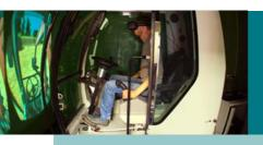
Safely controlling 20 tons with virtual machines: driver's cabin with virtual reality visor for machine operators undergoing training in the building trades.
