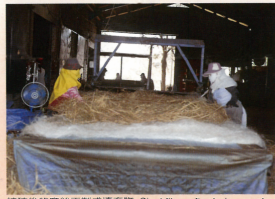
絞碎後的麻絲正製成填充物 Sisal fiber after being crushed is manufactured as mattress fillers
